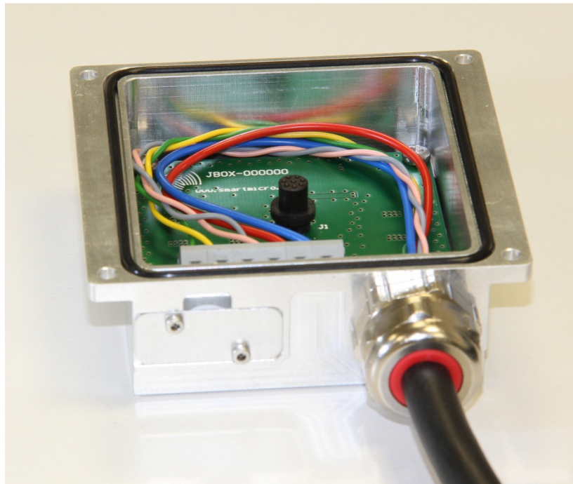
Figure 1: Junction Box JBOX-000000 with attached Lapp cable
