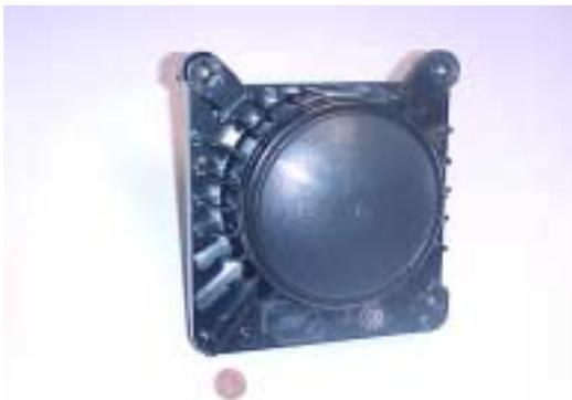
Figure 1: Photograph of the new radar sensor, a German Pfennig coin ( $\varnothing$  16,5 mm) illustrates the dimensions of the sensor
