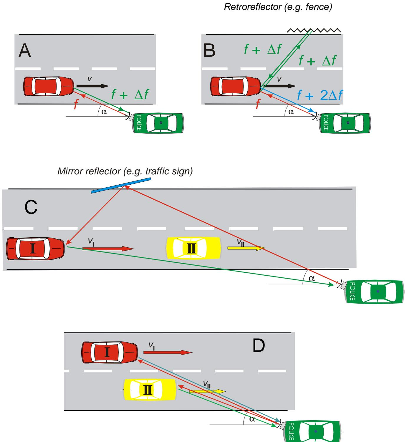
Figure 2: Situation with traffic radar used in Europe; part A shows the standard situation of a speed measurement, part B illustrates double reflection, C cracked beam reflection and D the situation of two vehicles hit by the beam at the same time (details see text above).
