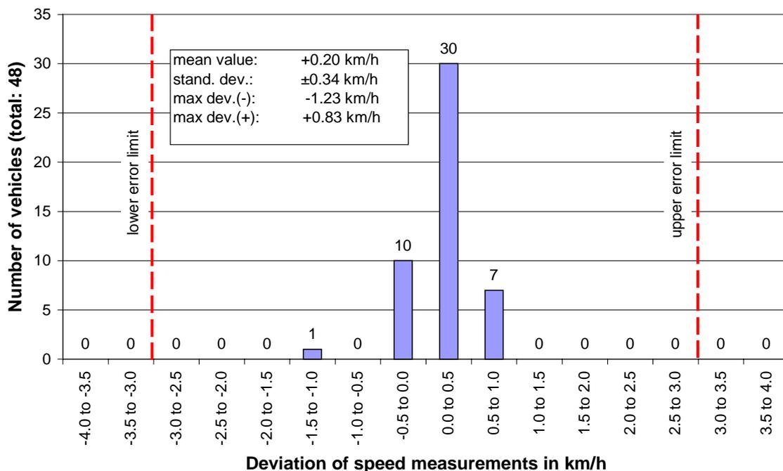
Figure 4: Comparison of the speed values measured by the new radar sensor with those measured by the PTB reference system.
