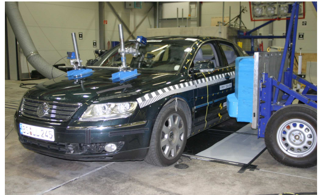
Figure 9. Phaeton just before real crash in a crash facility using IIHS barrier.
