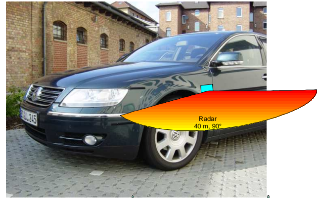
Figure 3. Volkswagen Phaeton equipped with the pre-crash recognition system and actuators.
