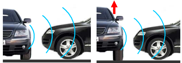
Figure 6. Phaeton before (left figure) and after lifting up the body (right figure).
