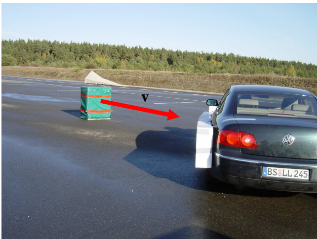
Figure 8. Pre-Crash-Evaluation of the equipped Phaeton using a dynamic collision object (green cuboid).
