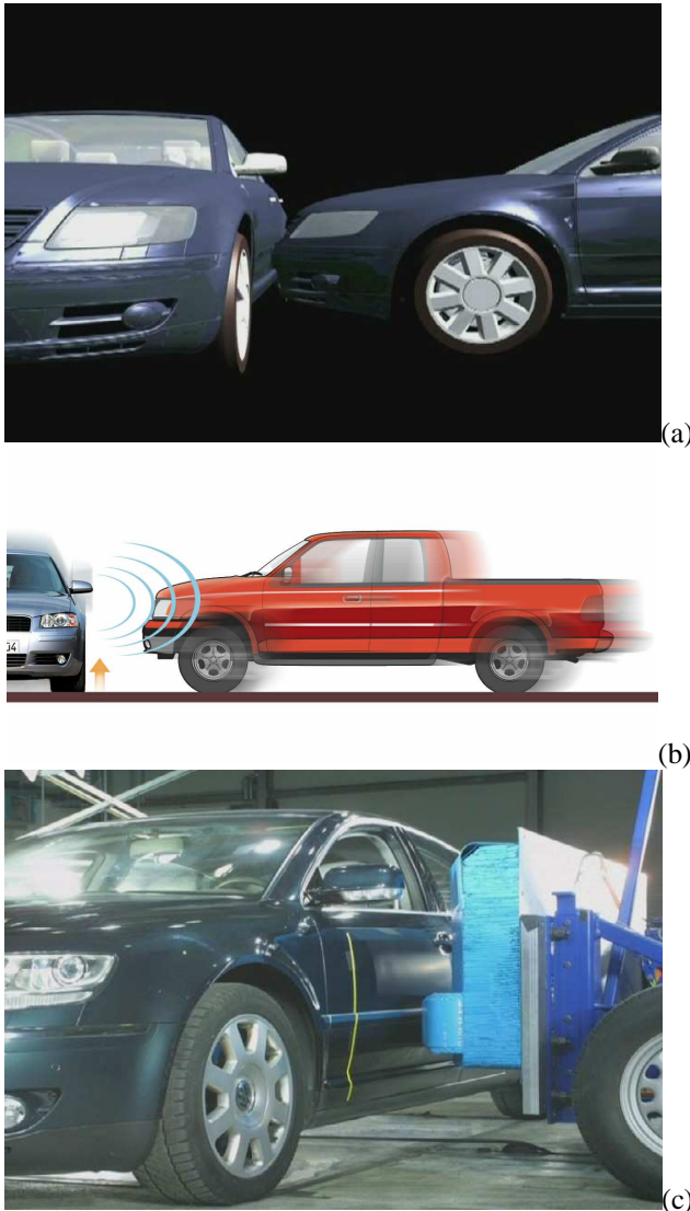
Figure 2. Bumper heights of different vehicles: (a) passenger vs. passenger car; (b) SUV vs. passenger car; (c) SUV vs. passenger car (standardized crash-barrier).
