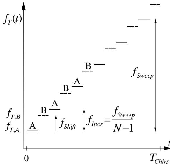
Figure 2: FMSK-2 Transmit Waveform
